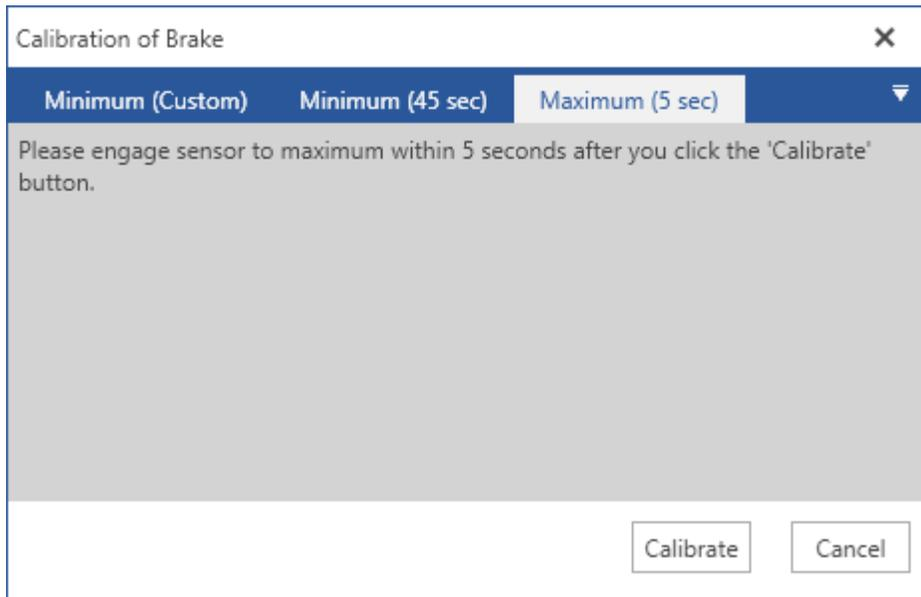
With “Maximum (5 sec)” calibration, you let the controller decide the maximum pedal pressure value. It does this by sensing the maximum pedal pressure in a 5 second window. Press the pedal with maximum braking force during these 5 seconds.
