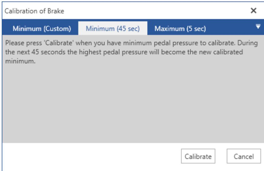
With “Minimum (45 sec)” calibration, you let the controller decide what will be the new minimum value. It does this by sensing the maximum pedal pressure in a 45 second window. Do not press the brake pedal after you have clicked calibrate – during this time window. This is a useful calibration when there is some noise or wiggling of sensor value.
