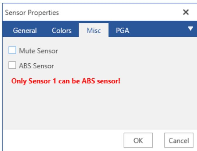
Check or uncheck "ABS Sensor" and click OK to set the abs.
